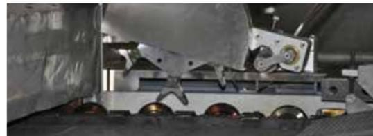
■ **Infrared sensor to read the stone plates' temperature at oven infeed**
